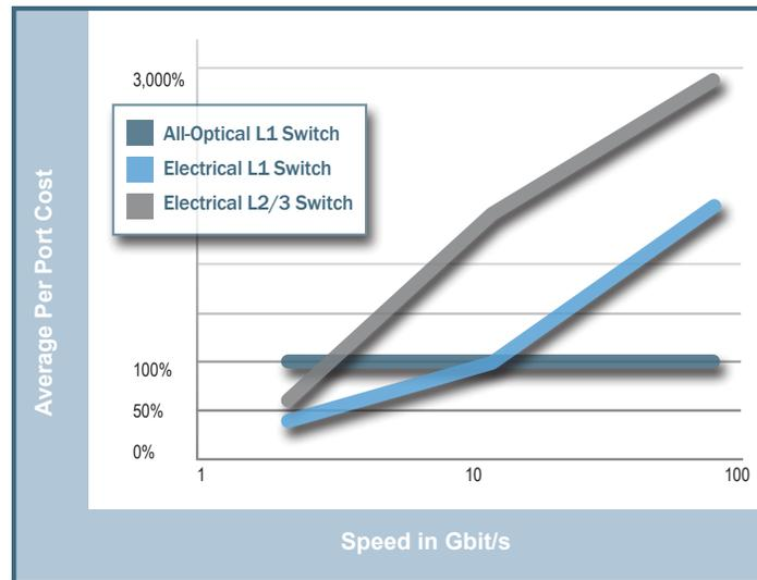
Figure 2. Average cost based on increase in speed.
