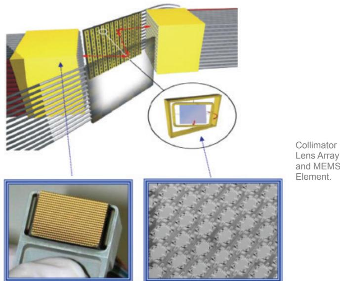
Figure 1. 320 x 320 3D MEMS Optical Switching.
