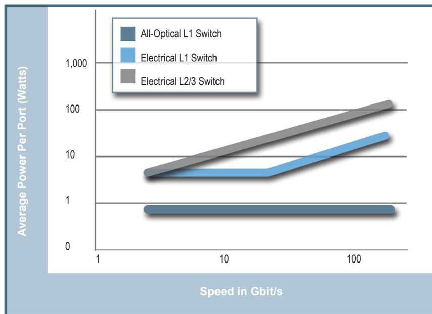
Figure 4. Average power based on increase in speed.
